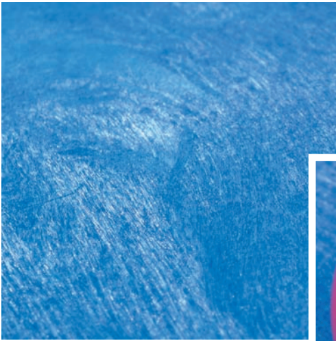
Swirled surface on plastic part in application where surface appearance is not critical.
