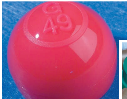
Class A surface with no swirling or sink marks.
